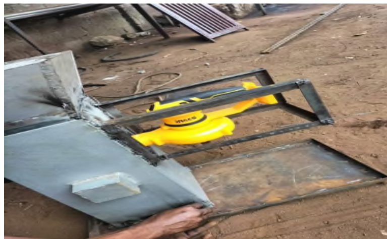
Figure 5: Automated fish feeding machine powered by a blower
