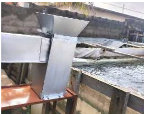
Figure 7: Developed automated fish feeding machine
